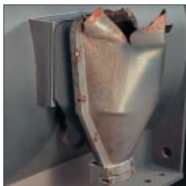
Standard 6 kV terminal box with opened relief joint
