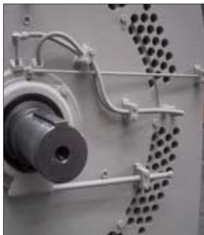
Antifriction bearing with lubricator and grease drain
