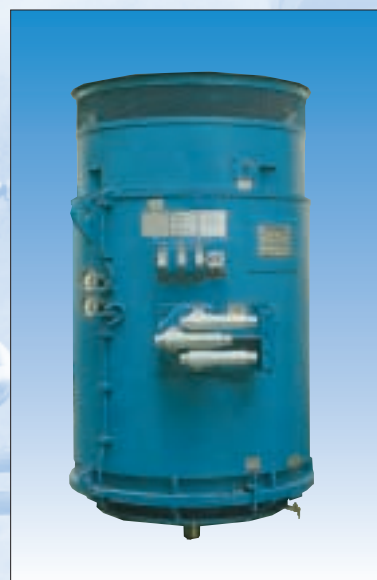
Pump drive, 600 kW, 6 kV, 2-pole, IM V1, connection via cable plugs
