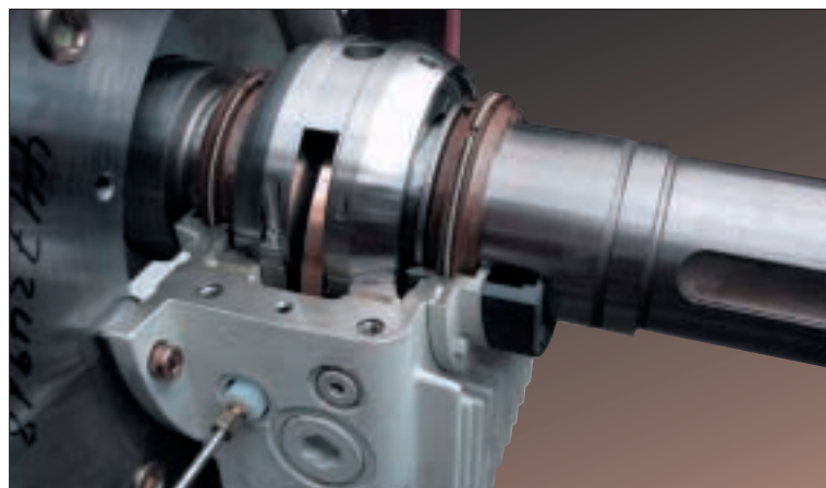
Sleeve bearing with ring oiler
