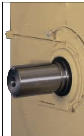
Antifriction bearing with lubricator and grease drain
