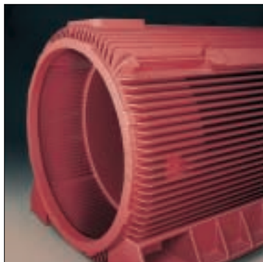
Casting of a size 560 frame
