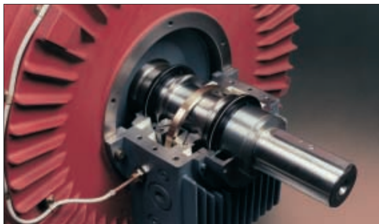
Self-lubricated sleeve bearing
