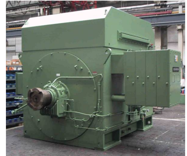
NDE with square-tooth clutch for drive by pony motor (turning gear)
