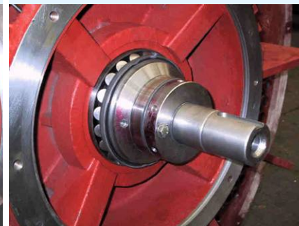
NDE with self-aligning roller thrust bearing
