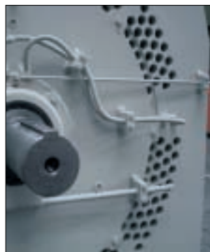
Anti-friction bearing with lubricator and grease drain
