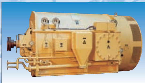
Drive for pipeline oil pump, Exd(e) IIA T3, 2, 600 kW, 6 kV, 2-pole; bearings with force-feed lubrication
